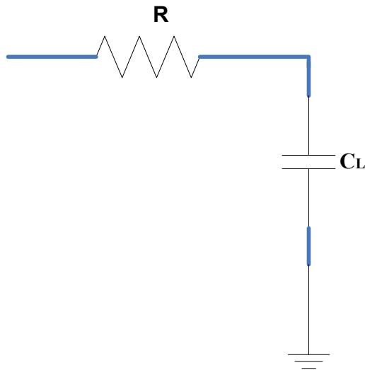
$$R = R_{\square} (L/W) = 0,08 \Omega/\square \cdot (1\text{cm}/3,6\mu\text{m}) = 222 \Omega$$
